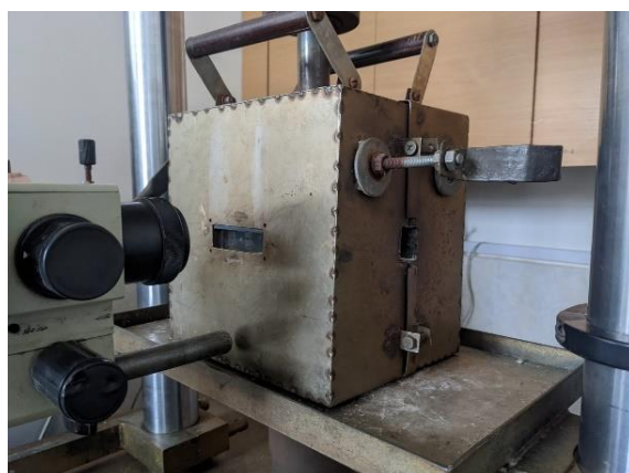
Figure 3. Thermochamber of the STM-100 test complex for determining the strength of VSt3ps steel at high temperatures
