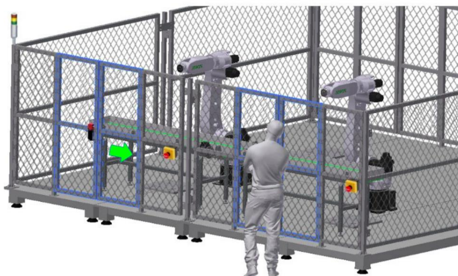
Figure 2. Protective fencing in robotic technologies, including collaborative ones
