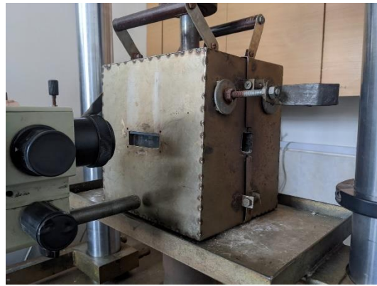
Figure 1. Thermochamber of the STM-100 test complex for determining the strength of VSt3ps steel at high temperatures
