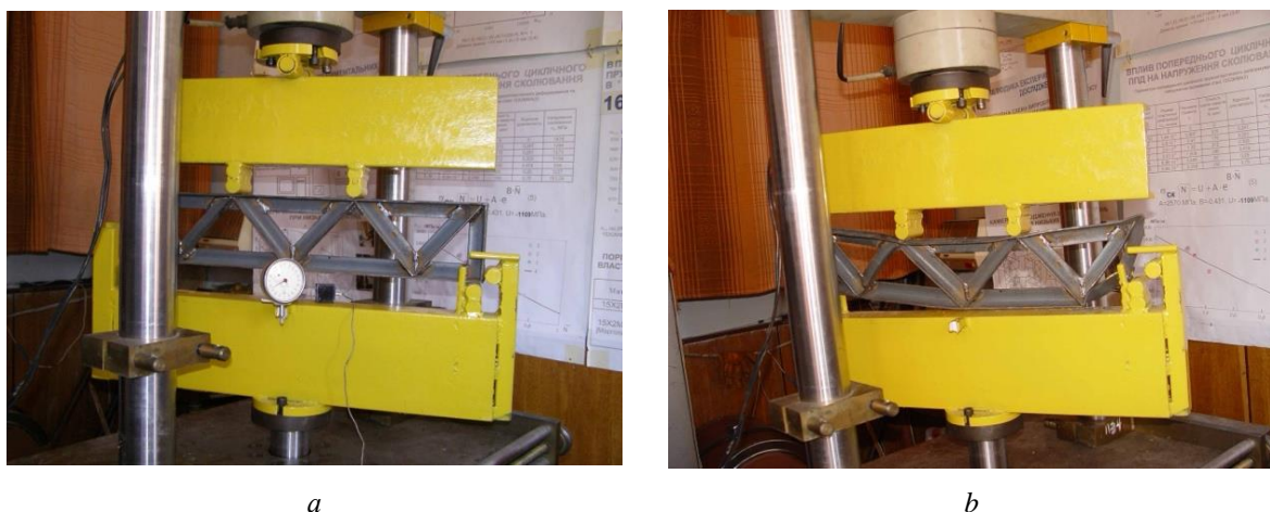
Figure 5. Sample of a welded truss on the STM-100 test complex before loading ( a ) and after fracture ( b )
