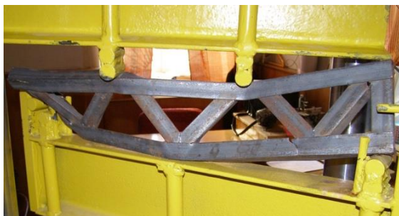
Figure 8. Physical model after fatigue failure
