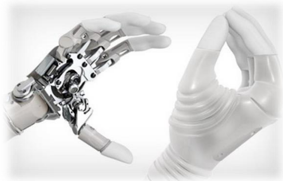
Figure 2. Appearance of the «Michelangelo hand» prosthesis [6, 7].
