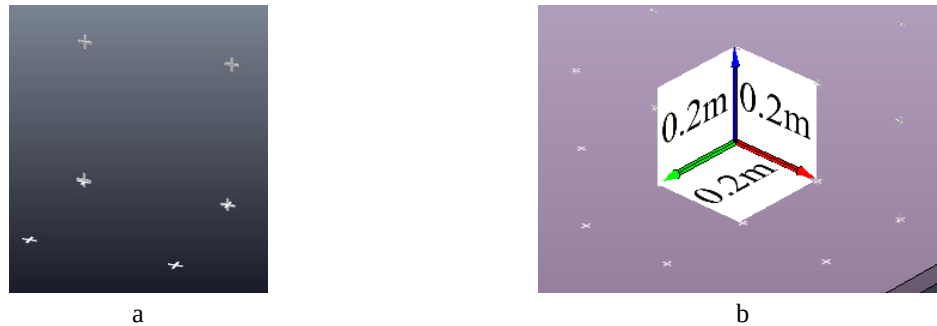
Figure 6. Dimensional vertical and horizontal parts of the grid (or) and dimensional cube (b) for enabling the verification of the actual dimensions of the operating areas
