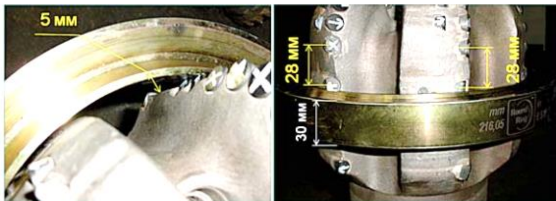
Figure 2. Control by 216,05 Round Ring™ gauge (nominal external diameter of the drill bit is 215,99 mm (8 ½ “), Round Ring™ gauge's height – 30 mm)
