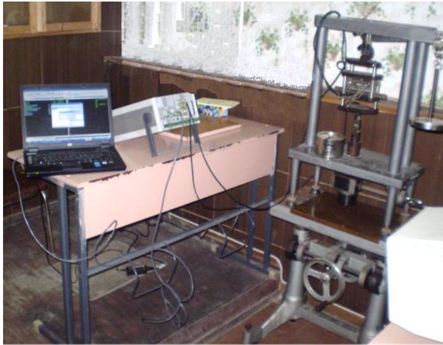
Figure 1. Strain gauge calibration at universal press UP-8
